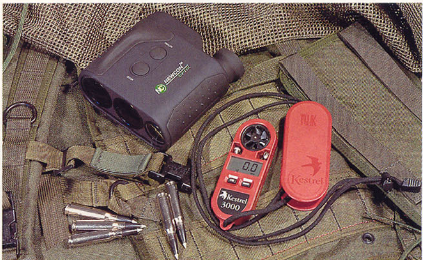
A compact unit, its small size can be noted here next to a Kestrel 3000 wind meter. Weight of the LRM 1500 is less than a pound.
